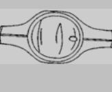
The venerable Ford 9 inch is both readily available and strong. Later models have bigger axle tubes and stronger housings. It was a standard under 1966-82 F-150s and Broncos. It also came on many vans and the Lincoln Versailles (a popular axle for swapping because of the Lincoln version of disc brakes with parking brake).
